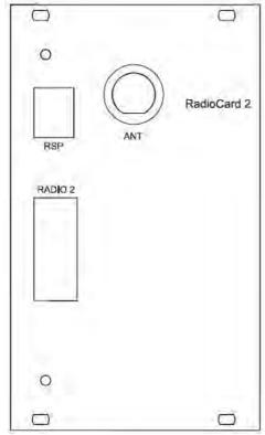
RSP – Radio serial port for programming without CPM (radio repeater stations), and for debugging.
